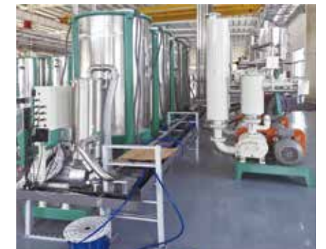
集中供料系统 Centralized feeding system
